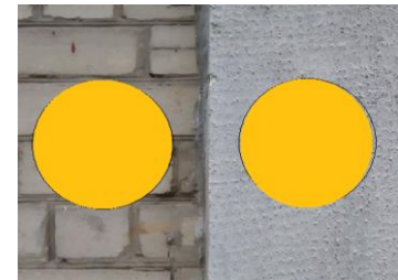
Fig.2. The scheme of scanning of a surface of a brick wall and a heater by a pyrometer with the laser pointer
